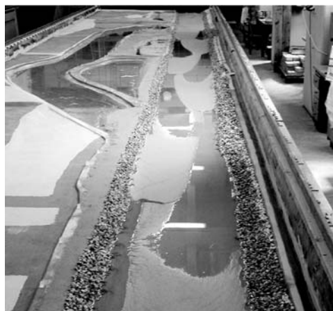
Figure 3. Development of alternate bars in the physical model at the bed-forming discharge.
